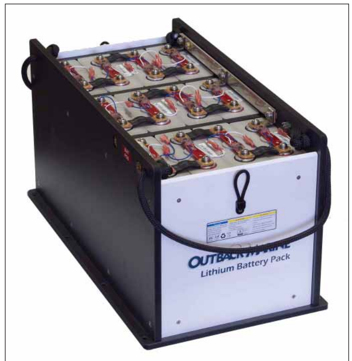
Lithium Iron Phosphate batteries have become the battery of choice for sailing catamaran owners who desire light weight and flexible charging performance. This 12 volt 540 AH battery is shown without top cover.
