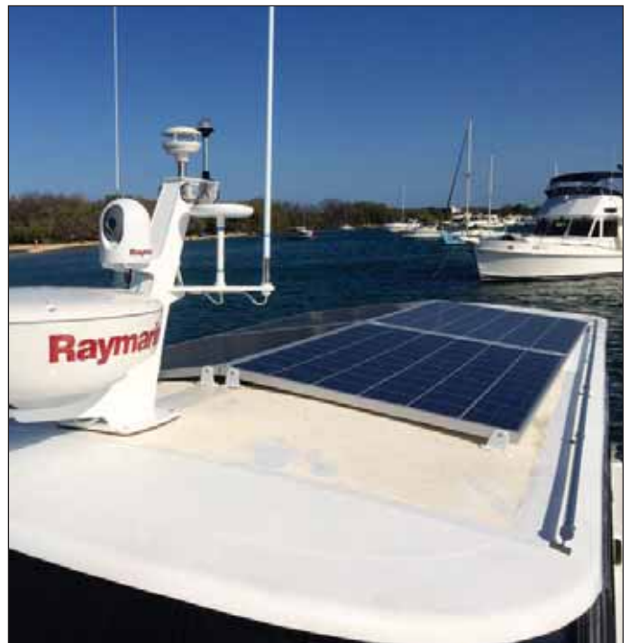
Solar panels are an effective means of energy generation for a cruising vessel. In this case, 1000 watts of solar has enough charging capacity to meet the daily electrical load including refrigeration and hot water heating.
