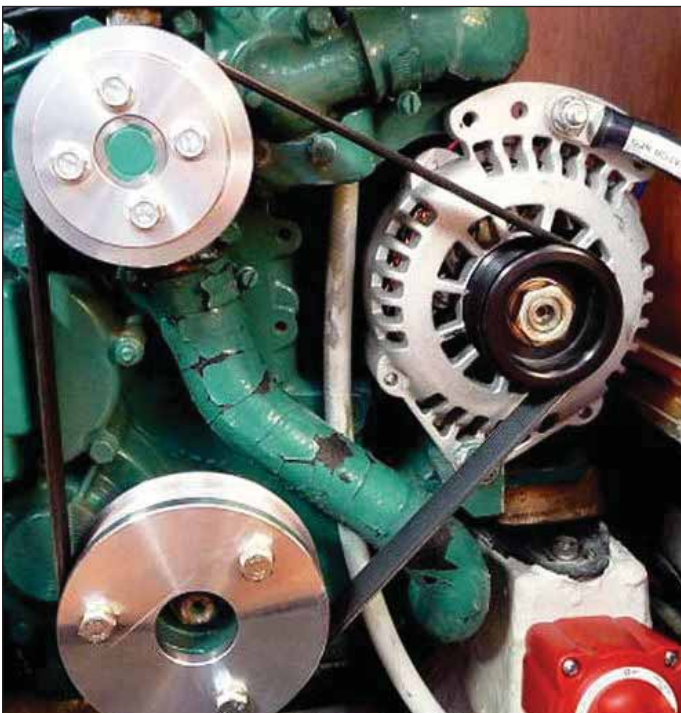
Replacing the standard engine alternator with a high output model can significantly reduce engine run time for battery charging at anchor. This unit is fitted with a high power capacity serpentine belt conversion kit.
