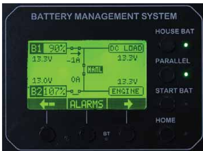
A graphic display gives a true representation of the electrical system status.
