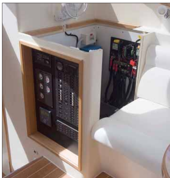
An electrical system cabinet on a Lightwave 38 sailing catamaran houses the electrical panels, Type 3 DCD Board, Inverter Charger and Solar Regulator. The DCD board is central to most heavy current devices.
