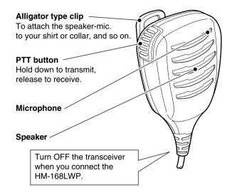
**NEVER** immerse the connector in water. If the connector becomes wet, be sure to dry it **BEFORE** connecting it to the transceiver.
