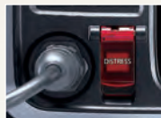
Distress button with a spring-loaded cover
