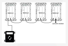
batteries; cannot mix; The matching address must select battery1 as the host, and long press and hold its reset button for 10s. Cannot select and press the reset button of other slave batteries. This step is particularly important as improper operation may result in battery networking failure.
