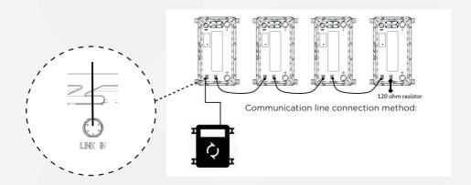
For normal battery operation, the CAN bus function is not mandatory. The battery can automatically operate and protect itself; it does not require any CAN bus communication or external devices (such as external controllers) or other CAN bus connected batteries to operate. Retain the two black covers installed on the two M12 connectors to protect them from environmental influences when not in use.
